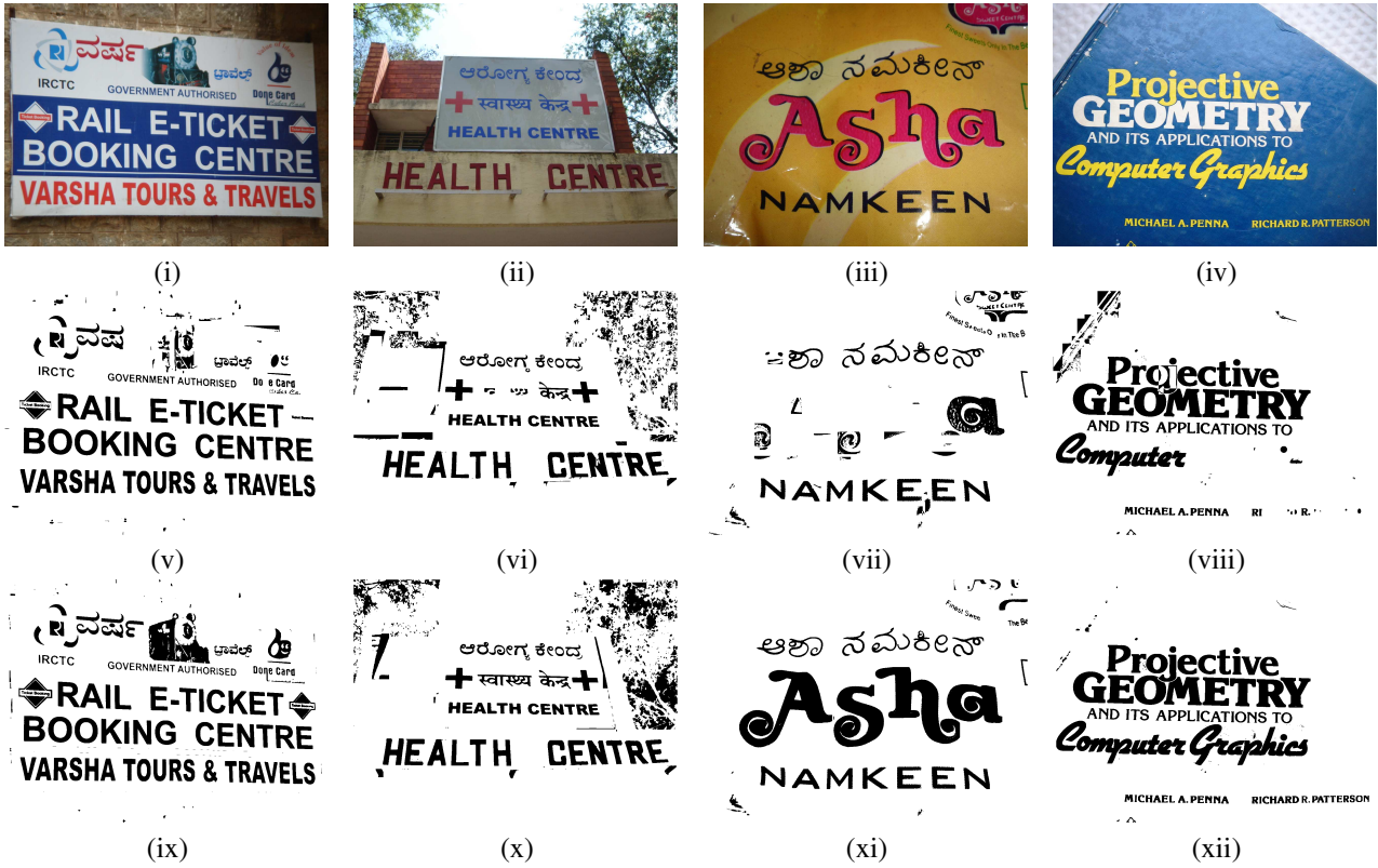
Figure 4. (i - iv): Input images having graphic objects, inverse text, multiple scripts, complex backgrounds and cursive letters. (v - viii): The corresponding binary outputs obtained using the method proposed in [7]. Clearly, the method is sensitive to background objects since it relies on the edge information to locate CCs. It also invokes script-dependent characteristics and works well only for isolated Roman letters. (ix - xii): Binarized output images obtained with the proposed method. Color segmentation provides robustness to background complexity as well as independence to script.
