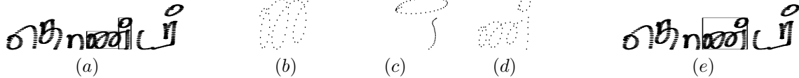
Fig. 4. Correction of over-segmentation. (a) Fourth symbol is split into two by DOS. (b) This Stroke group has a low posterior probability and is suspected to be a part of a symbol. (c) The second split part of the symbol also has low posterior probability. (d) Merged symbol has higher likelihood. (e) Correctly segmented word.
