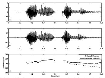
Fig. 6. Affirmative to Interrogative conversion using pitch modification. (a) Waveform of an affirmative sentence. (b) Synthesized Interrogative sentence (c) Pitch contours of (a) and (b).
