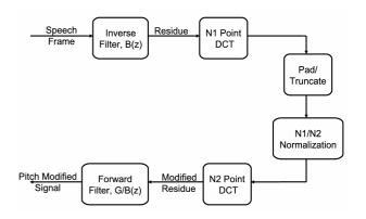
Fig. 1. Block diagram of pitch modification using DCT/IDCT via PMVDR spectral modelling.
