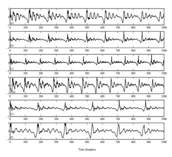
Fig. 2. (a) Few frames of an utterance /A/ and (b) its excitation.(c) Excitation in (b) modified for a pitch increase factor of 1.3. (d) Signal resynthesized by forward filtering the signal in (c) using 1/B(z) coefficients. (e) Excitation in (b) modified for a pitch decrease factor of 0.7. (f) Signal resynthesized by forward filtering the signal in (c)
