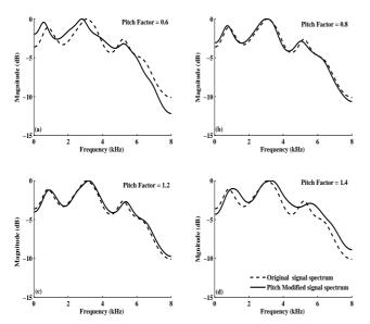
Fig. 3. PMVDR Bauer spectra of the original signal overlapped with those of the modified signals for pitch modification factors a) 0.6 (b) 0.8 (c) 1.2 (d) 1.4.
