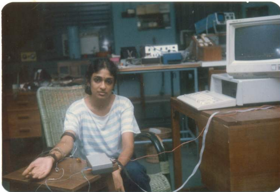
Fig.3.3. Recording of CNAP in progress from elbow site - median nerve stimulation at wrist.
