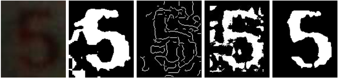
Figure 7: Segmentation of a sample word image from ICDAR 2003 dataset. (a) Original image. (b) Output of Otsu's method [1]. (c) Edges by Canny's method [3]. (d) Binarized output of Niblack's method [4]. (e) Output of MAPS technique using Min-Max method for segmentation and Max-flow algorithm for classification.
