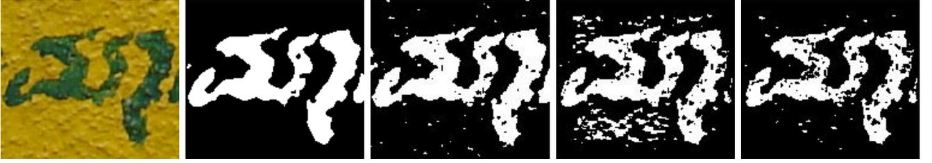
**Figure 4: Comparison of outputs of different binarization techniques. (a) A sample image. (b) Classification of pixels using energy minimization function. (c) Otsu's global thresholding. (d) Niblack's local thresholding. (e) Sauvola's and Pietäikinen's local thresholding.**
