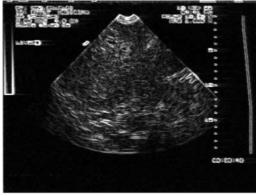
Fig. 1. Edge Detected Ultrasound Image using Sobel operator.
