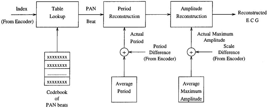
FIG. 2. Block schematic of the decoder.
