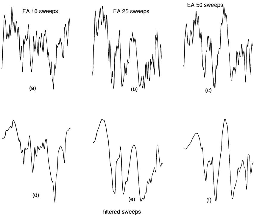
**FIG. 8.** Comparison of filtered outputs with EA at different ensemble lengths for MLR data. (a–c) The ensemble averages. (d–f) The corresponding filtered sweeps.
