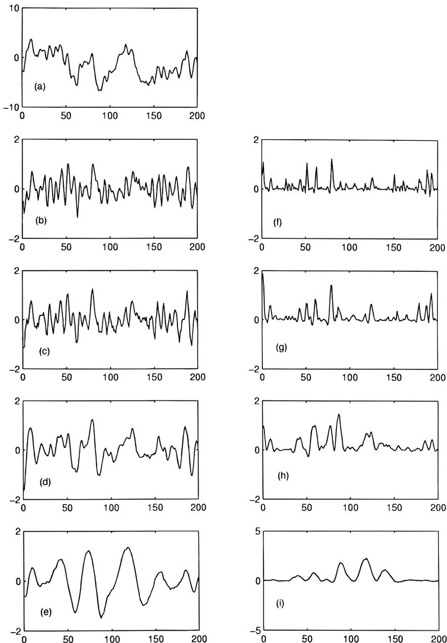
**FIG. 3.** Nonorthogonal decomposition of the signal and the correlation between its adjacent scales. (a) The signal. (b–e) Components at scales 1, 2, 3, and 4, respectively. (f–i) Correlation between scales 0 and 1, 1 and 2, 2 and 3, and 3 and 4, respectively. [X axis in all cases, Sample No.; Y axis in b–e, amplitude in relative units; in f–i, correlation in relative units.]
