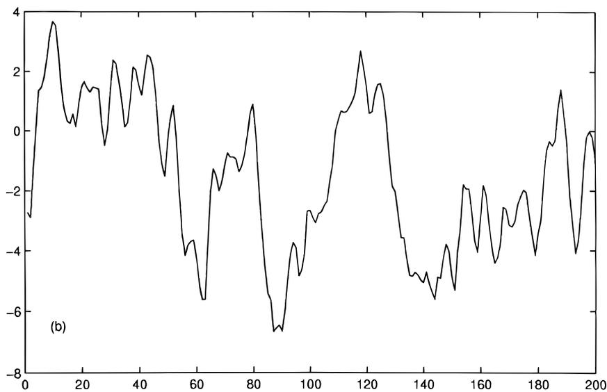
**FIG. 1.** Typical auditory middle latency response. (a) Single sweep. (b) Ensemble average of 30 sweeps. [X axis, Sample No.; Y axis, amplitude in relative units.]
