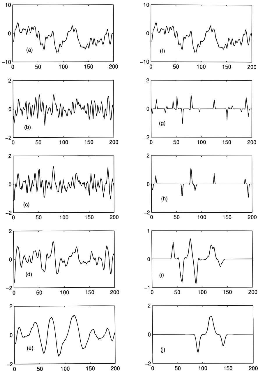
**FIG. 5.** Wavelet coefficients using UDWT at different scales before and after nonlinear filtering using Gaussian functions. (a, f) Original signal. (b–e) The wavelet decompositions at scales 1, 2, 3, and 4, respectively. (g–j) The corresponding filtered decompositions. [X axis, Sample No.; Y-axis; amplitude in relative units.]
