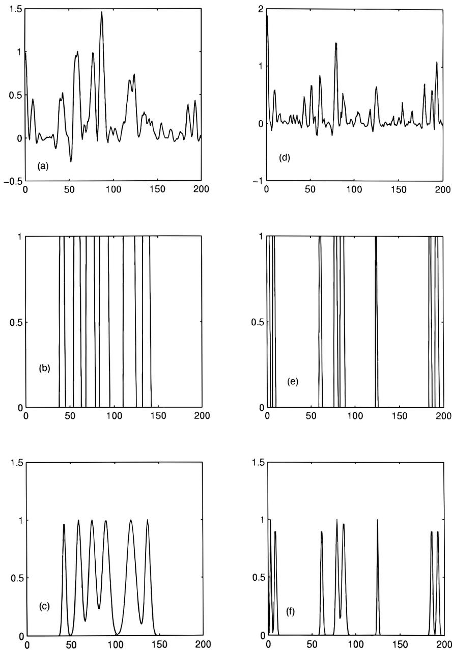
**FIG. 4.** Wavelet coefficients retained using binary mask and Gaussian mask. (a) Correlation between scales 2 and 3, (b) Binary mask obtained using selective filtering. (c) Gaussian mask using our method. (d–f) Corresponding figures for correlation between scales 3 and 4. [X axis in all cases, Sample No.; Y axis in a and d, correlation in relative units; in b, c, e, and f), magnitude in relative units.
