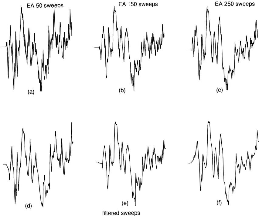
**FIG. 9.** Comparison of filtered outputs with EA at different ensemble lengths for AEP data. (a–c) The ensemble averages. (d–f) The corresponding filtered sweeps.
