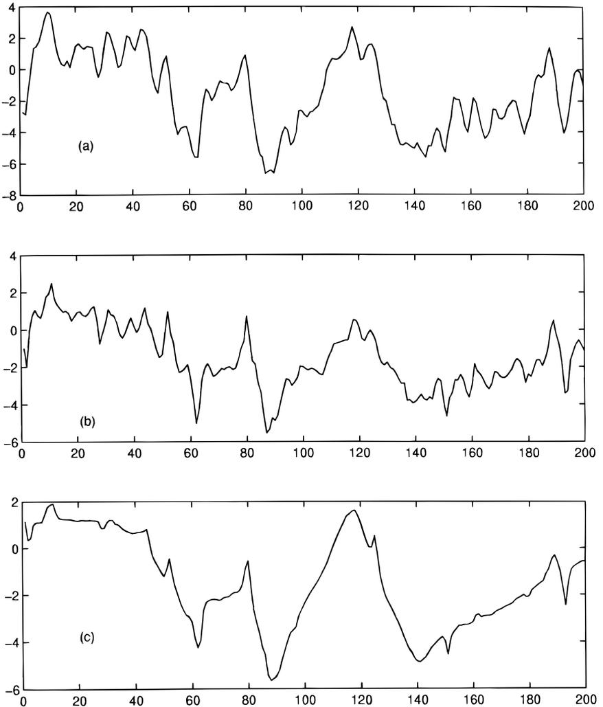
**FIG. 6.** Comparison of outputs obtained using binary and Gaussian masks. (a) Middle latency AEP shown in Fig. 1a. (b) Filtered output obtained using binary masks. (c) Output obtained using Gaussian masks. [X axis, Sample No.; Y axis, amplitude in relative units.]
