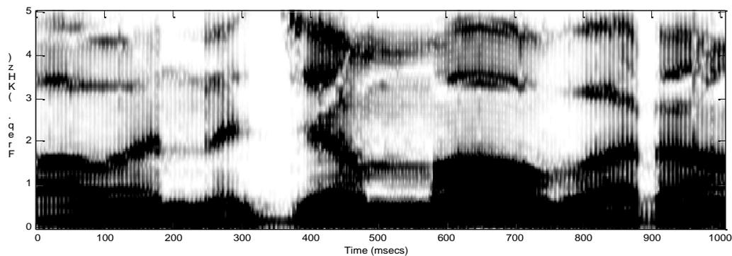
Fig. 6(b) Spectrogram of the utterance after pitch modification by a factor of 1.2.
