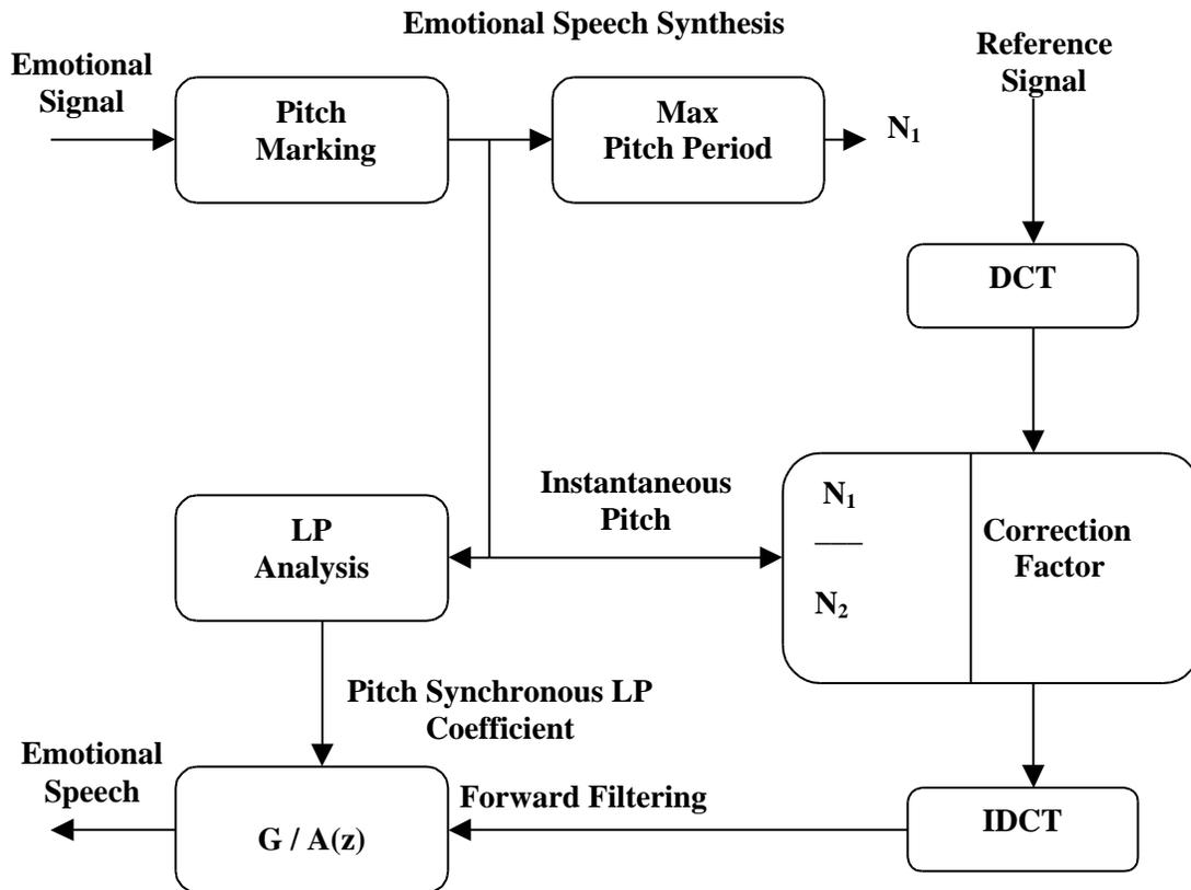
Fig. 4. Block Schematic of Emotional Speech Synthesis
