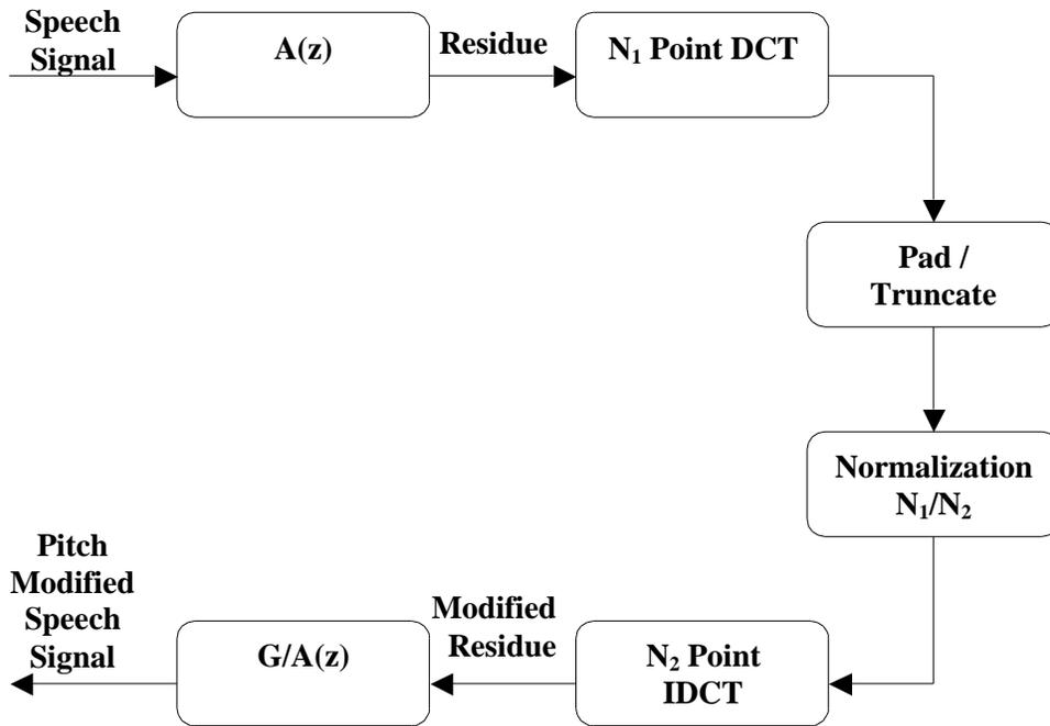
Fig. 5. Block Schematic of Pitch Modification System
