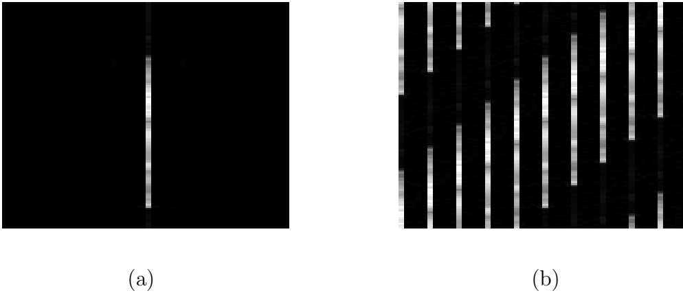
Figure 3.4: Typical y - f maps obtained from k -space data acquisition for acceleration factor 5 using : (a) Densely sampled low k -space (Training data) (b) Sparsely sampled full k -space (Actual data)
